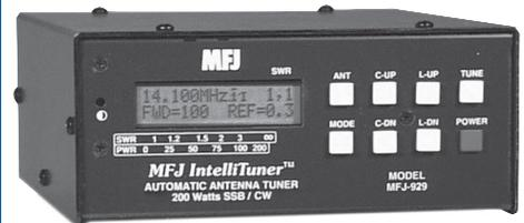
The MFJ-929 IntelliTuner™ lets you automatically tune any coax fed or random wire antenna 1.8-30 MHz at full 200 Watts SSB/CW. It can match 6-1600 Ohms (SWR up to 32:1). You get a digital SWR/Wattmeter with backlit LCD and an antenna switch for two antennas. Requires 12-15 VDC at 1A and appropriate interface cable. **Sale!**
