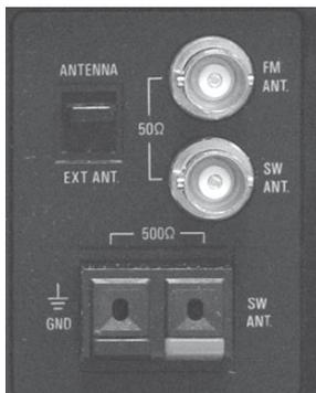
Switchable BNC jacks are provided for FM and shortwave antennas. High impedance (500 ohm) terminals are provided for simple shortwave wire antennas. There is also a mini jack available for the AM and longwave bands.
